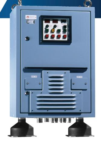
This solid-state 60 Hz to 400 Hz Converter is capable supplying a nominal consumer load up to full power of 5kW/kVA with a power factor of 0.8 lagging to 1.0 to 0.8 leading continuously. The Unit is able to supply an overload up to 130% for 3 min and it comprises a short-circuit protection with constant current behavior, enabling a short-circuit current of approx. 2 x Inom for 30 s during load failure conditions.
